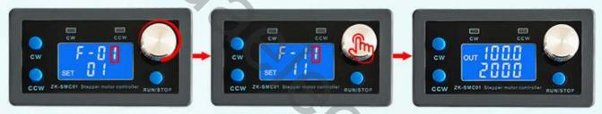
In the menu setting interface, adjust the rotary encoder to change the parameter codes F-01~F-13.
